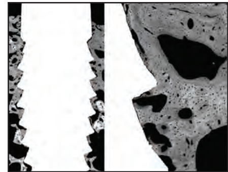
Figure 3 Scanning electron photomicrograph (backscattered electron imaging model) of bone integration of an experimental implant at 3 months (uncovering). Left: Overview (collage) of several images showing bone integration of the body of the implant as well as direct bone integration of the laser-micromachined collar. Right: Higher magnification of bone integration of the implant body. Thread pitch = 1 mm.
