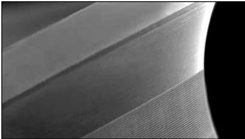
Microchannels viewed using scanning electron microscopy (SEM) at 1000X
